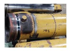
For this application, the hydraulic cylinders provided the bending force on large diameter pipes (up to 36" diameter) as it was fed through the bending carriage. Over a short period of time, the inadequate cylinder design and application forces created hydraulic leaks at the head glands. Consequently this resulted in equipment removal from standing projects as well as replacement of the cylinders, both costly procedures.
