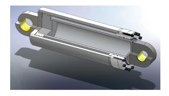
Upon receiving the first batch of cylinders, each cylinder was subject to reverse engineering to gain a full understanding of the defects inherent to the current design and application. New design modifications to the head gland, piston, and seal package were implemented to eliminate the leaking cylinder issues previously experienced.
